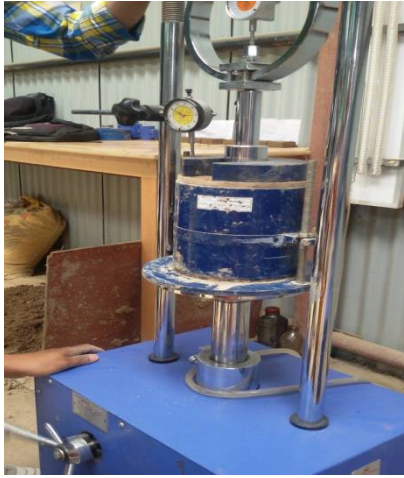
Fig. 2: CBR test being conducted in the laboratory
